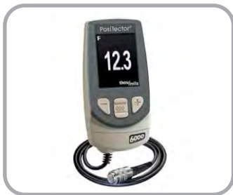
COATING THICKNESS TESTING
